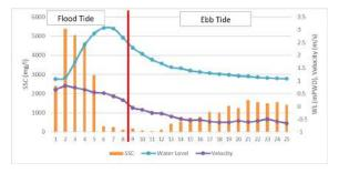
Figure 3: Sediment concentration in a full tidal cycle at Bhabadah
