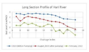
Figure 6: Long Section Profile of Hari River before and after pumping
